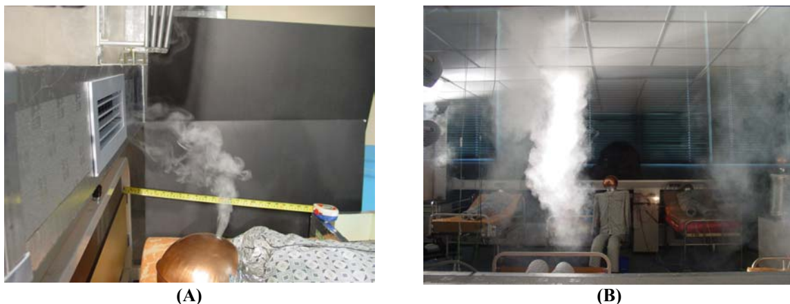
Figure 1. Smoke visualization of the exhaust (A) and supply (B) air streams in the full-scale test room at HKU.
